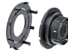
In order to counteract the non-uniform distribution of warm air in multi-duct systems with several air outlets, we have developed innovative air flow regulating elements that are simply clipped into the hose connection fitting of the air outlet. The regulating elements reduce the flow cross section as needed and thereby decrease the emerging air flow. Available for fitting diameters 60, 75 and 90 mm.
